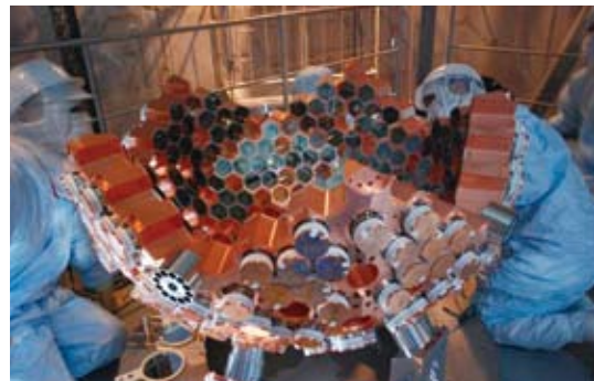
XMASS detector during construction ©ICRR
